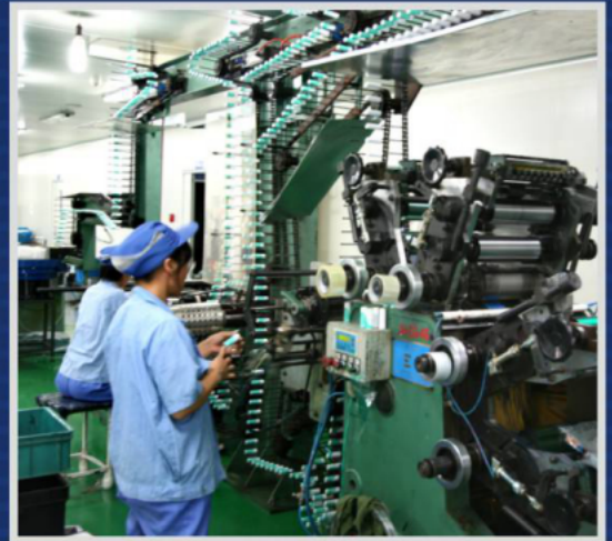
Automatic printer for aluminium bottles
