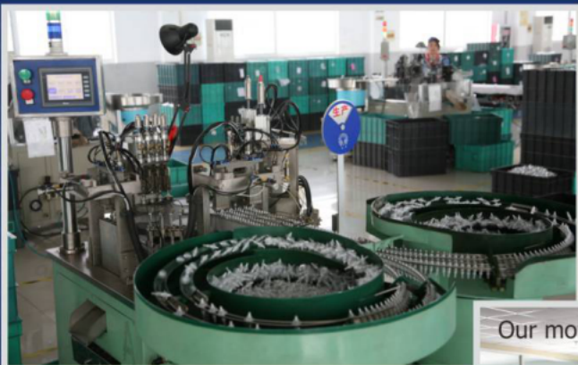
All spray pumps are tested by vacuum test machines by 100% during production
